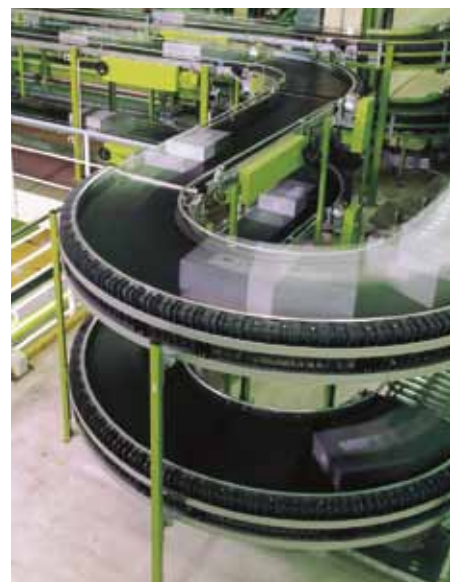
Curved conveyor in a distribution centre.
