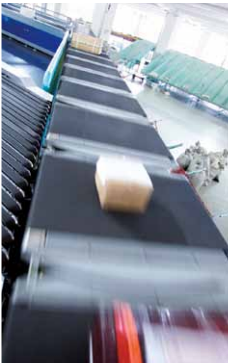
Lateral sorter in a distribution centre. The high acceleration requires the belt surface to have an extremely high coefficient of friction.
