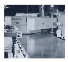
Accumulation belts are used when collecting conveyed goods behind a barrier or when sliding onto or off a belt. The particularly stiff design of the belts ensures level conveying in larger belt widths. So pushing unit goods on or off from the side is no problem at all.
