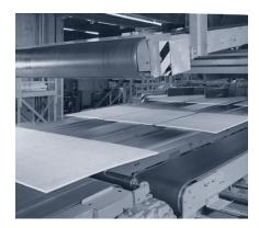
Antistatic Siegling Transilon belts are equipped with an electrically conductive static inhibitor that is abrasion-protected and embedded in the belt.
