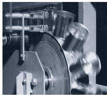
Siegling Transilon NA belts are produced without an electrically conductive antistatic element. Tested according to ISO 21178 the electrical surface resistance  $R_{Di}$  is more than 3 x 10<sup>8</sup>  $\Omega$ .
