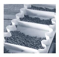
Conveyor belts equipped with profiles are used for the inclined conveying of bulk goods and small items.
