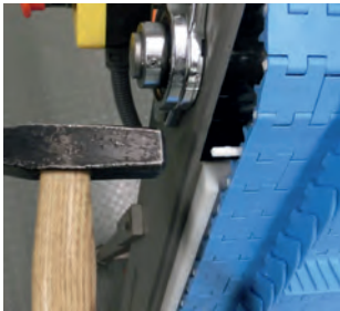
3 Gently tap its head into retaining position
